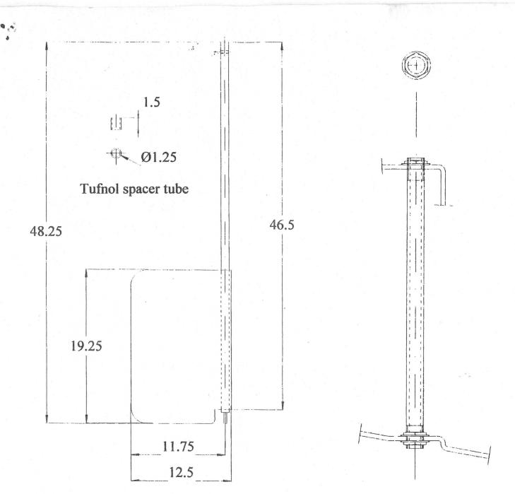
Rudder assembly as fitted to Mk III Silhouettes, not as shown in general arrangement drawing Sheet No 5.
