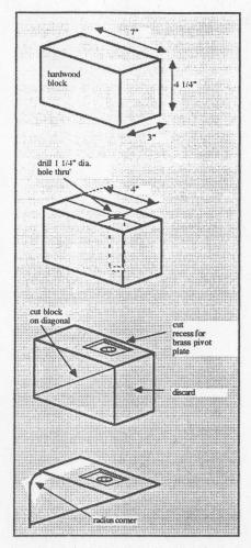
worth making it thicker than the original - say 1/4" so as to give a greater bearing surface against the rudder stock. The recess for the plate is easily gauged out so that the plate fits flush with the surface.
